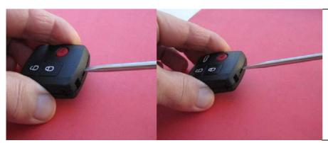
Use small flat screw-driver to open remote key on the split line separate it into two parts and remove worn key pad.
