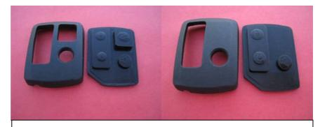
Place top part of hard shell with fitted new pad over the bottom part and press firmly till remote closes
